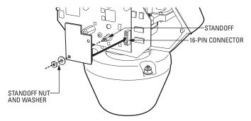
Figure 3. Installing the TXB-V into the Esprit
